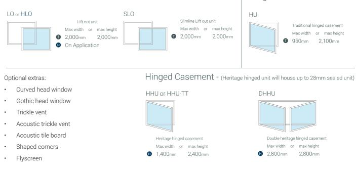
All windows are supplied fully assembled and ready to install. Units comprise of an aluminium outer frame joined to a seasoned hardwood timber surround.
